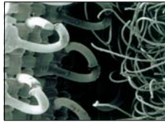
Fig.1. Image of Velcro's hooks and loops (eyes)
