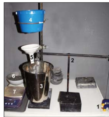
Fig. 1. Bench bond-strength tester. A controlled, increasing weight (stainless steel balls) pulls a wire, the end of which can be attached to bracket tie-wings, and various holding devices: 1. Sample tested (brackets bonded to a gold coin). 2. System of pulleys transmitting the force; 3. Container for fallen metal balls. 4 & 5. Sand-timer system working with steel balls. 6. Container for the latter. 7. Scale.
