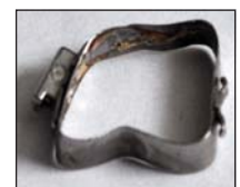
Fig. 2. Worn band, as removed
