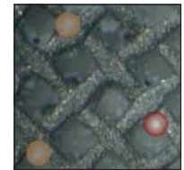
Fig. 2 b. Spacers even up the thickness of an adhesive
