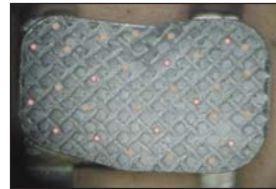
Fig. 2 a. Distribution of colored spacers in a photocured adhesive
