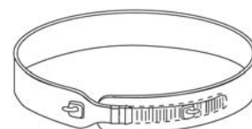
Fig. 1 Recent patent for molar bands. A strip of flexible material can be locked at each end of the strip
