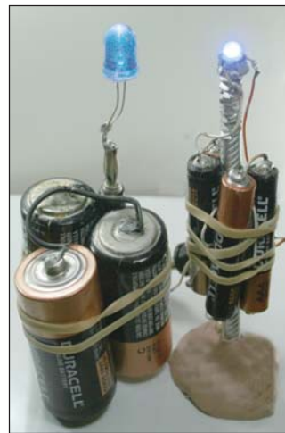
Fig. 7. Mounted LEDs: Observe the aluminum spike used as both heat sink and support
