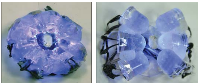
Fig. 12. Common LEDs arranged in a star-type configuration. a. Eight 3mm LEDs, glued; b. Six 10mm LEDs, free on wires.
