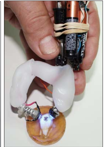
Fig. 14. ShapeLock allows any desired shape which can be quickly immobilized
