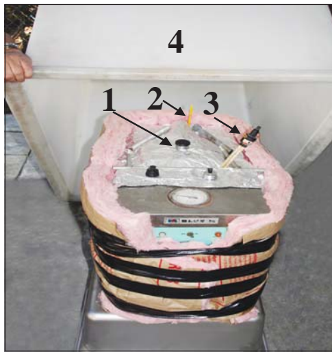
Fig. 4. Insulated oil bath containing pressure cooker 1. Regulator on the cooker's lid controlling steam escape. 2. Mercury thermometer. 3 Thermoregulator. 4. Plastic tank.
