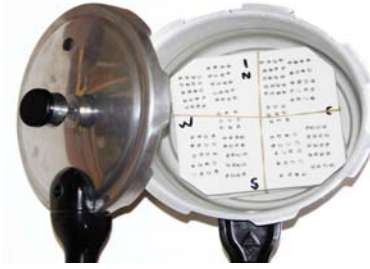
Fig. 2. Pressure cooker with brackets bonded on ceramic tiles
