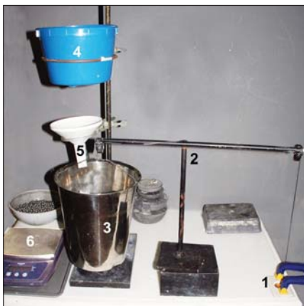
Fig. 1. Bench bond-strength tester. A controlled, increasing weight (stainless steel balls) pulls a wire attached to bonded brackets' tie-wings: 1. Sample tested., 2. System of pulleys transmitting the force.; 4, 5. Sand-timer system., 6. Scale.
