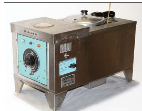
Fig. 3. Pressure cooker in the oil bath
