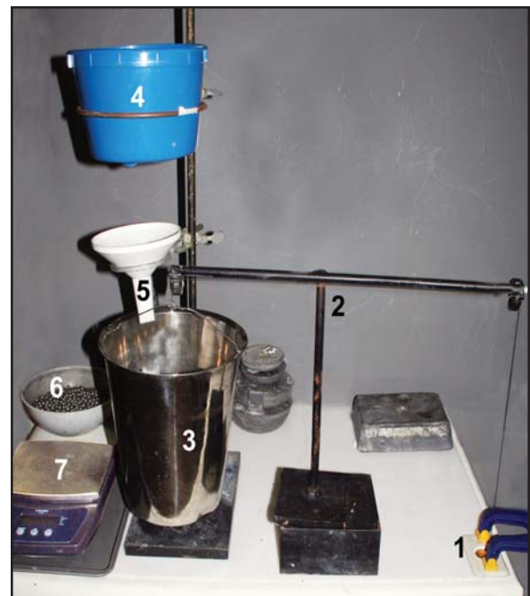
Fig. 1. Bench bond-strength tester. A controlled, increasing weight (stainless steel balls) pulls a wire, the end of which can be attached to bracket tie-wings, and various holding devices: 1. Sample tested (brackets bonded to a gold coin). 2. System of pulleys transmitting the force; 3. Container for fallen metal balls. 4, 5. Sand-timer system working with steel balls. 6. Container for the latter. 7. Scale.
