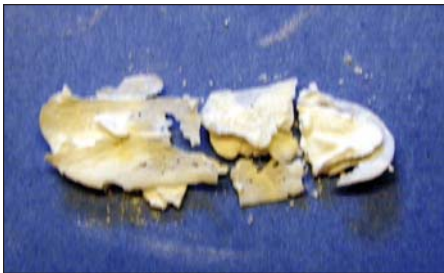
Fig. 6. The thin, friable film formed at the contact surface of the two composite blobs shown in Fig. 4 & 5
