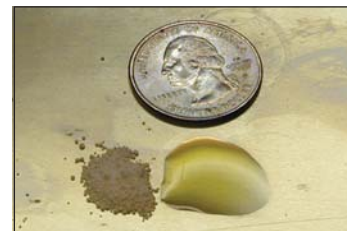
Fig. 2. Granules of benzoyl peroxide and a drop of N,N -dimethyl p -toluidine.
