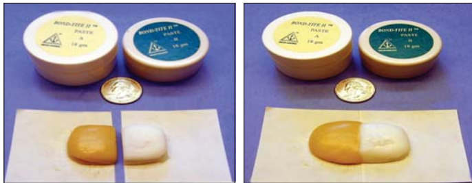
Fig. 4 & 5. Blobs of reactive pastes before (a) and after being pressed one against the other (b).
