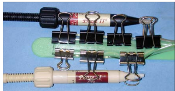
Fig. 7. A cut open Nalgene™ tube along with the screw syringes containing parts A and B of the adhesive Phase II
