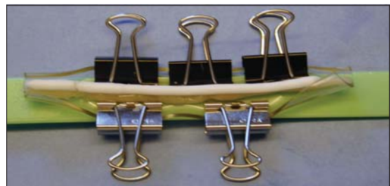
Fig. 9. Superimposed streaks of the adhesives Phase II laying on the cut open tube
