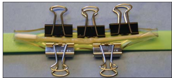
Fig. 8. A streak of the adhesives part A laying on the cut open tube having on it (right) a small amount of Part B.
