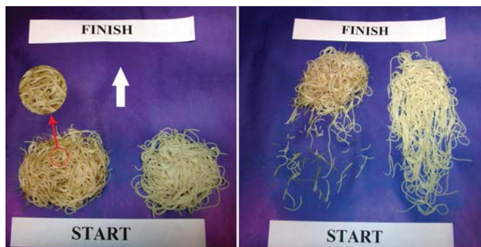
Fig. 4. An addition of dry spaghetti fragments (left piles) toughens a pile of boiled ones
