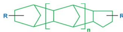
Fig.11 Long and planar polycyclic monomer in which R can be a methacrylic moiety.
