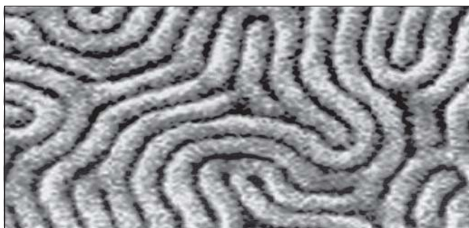
Fig.3. SEM image of top edges of thin sheets of polystyrene and polymethylmethacrylate
