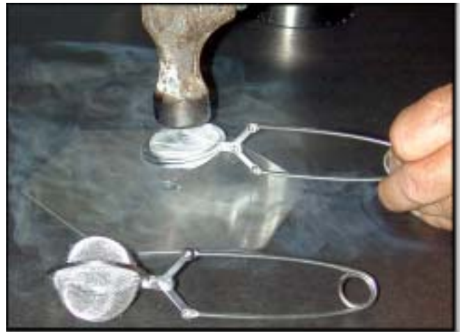
Fig. 2. Reduction of the deep-cooled plastic materials and a stainless steel tea basket
