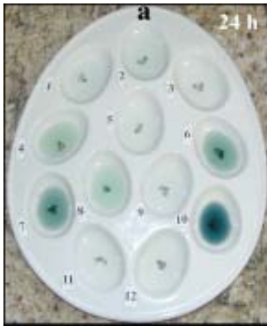
Twelve brands of brackets successively subjected to batches of 5% hydrochloric acid. a. After 24 h from the first addition. b. After 48 h since the spent acid has been replaced. c. After another 48 h since the last spent acid has been replaced.
