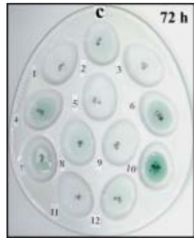
Twelve brands of brackets successively subjected to batches of 5% hydrochloric acid. a. After 24 h from the first addition. b. After 48 h since the spent acid has been replaced. c. After another 48 h since the last spent acid has been replaced.
