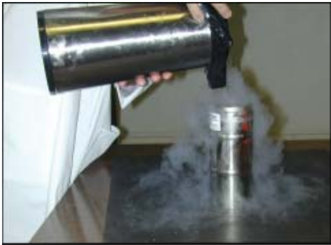
Fig. 1. Transfer of liquid nitrogen into a cryogenic container allowing the immersion of a steel tea-basket
