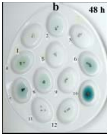
Twelve brands of brackets successively subjected to batches of 5% hydrochloric acid. a. After 24 h from the first addition. b. After 48 h since the spent acid has been replaced. c. After another 48 h since the last spent acid has been replaced.
